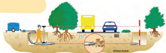
Impact Moling illustration (courtesy of TT-UK Ltd)
